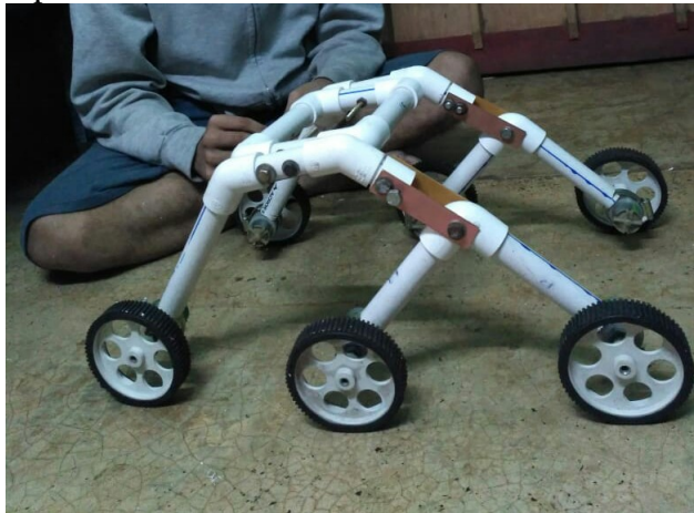
FIG 3: Rocker Bogie Mechanism for the model
