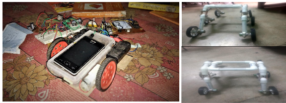
FIG 2: Test model with DTMF decoder circuit and cell-phone
